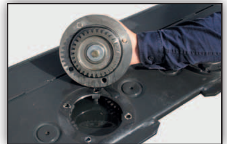
Individual top service hubs can be removed very quickly for easy maintenance.
