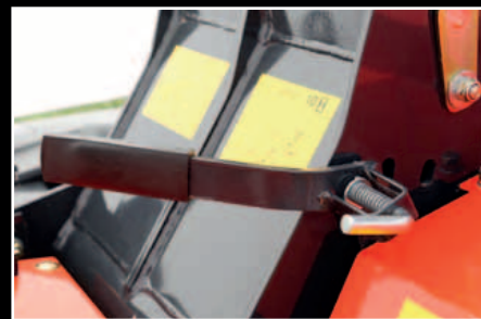
Easy adjustment of conditioning intensity – 3 different positions possible.
