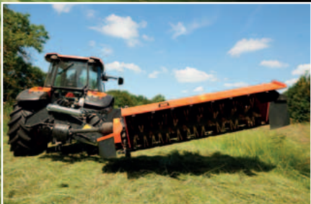
Lift on headland with ample clearance to existing swaths.
