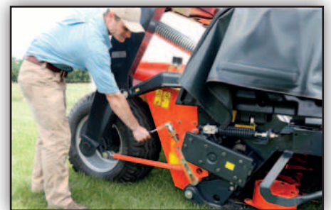
Easy adjustment of stubble height.
