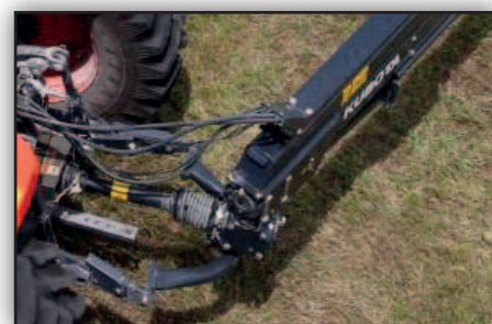
The swivel hitch headstock with reversible gearbox provides optimal manoeuvring ability.
