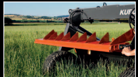
Dismount the two deflector doors and you are ready to mow.
