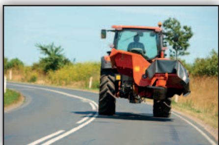
During transport the machine is folded hydraulically to a horizontal position well in behind the tractor, thus minimising transport width.
