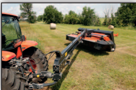
A lifting height of 50cm, ensures excellent ground clearance for transport and during headland turning.
