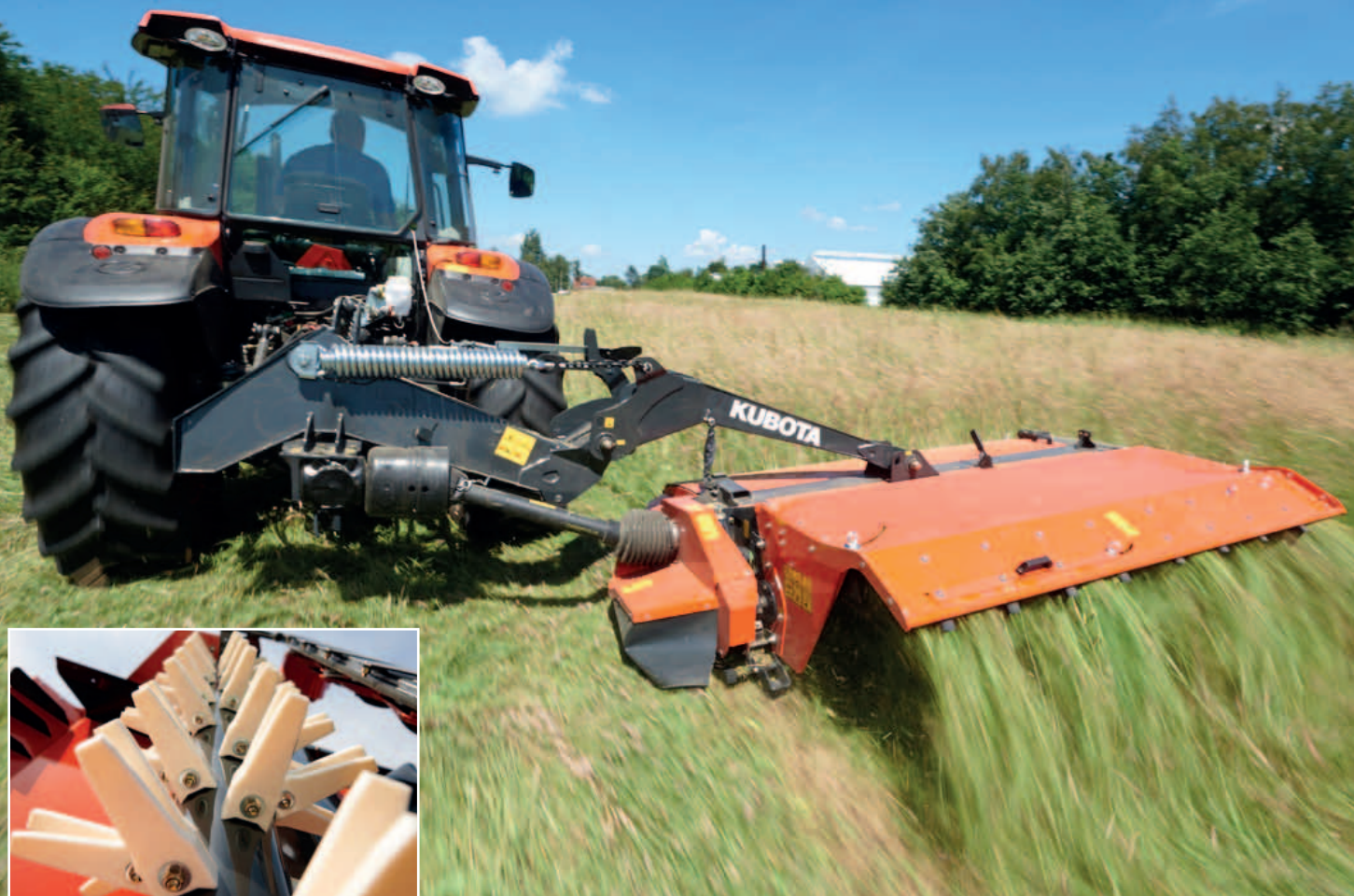
Effective 600/900 nylon tine conditioning.
