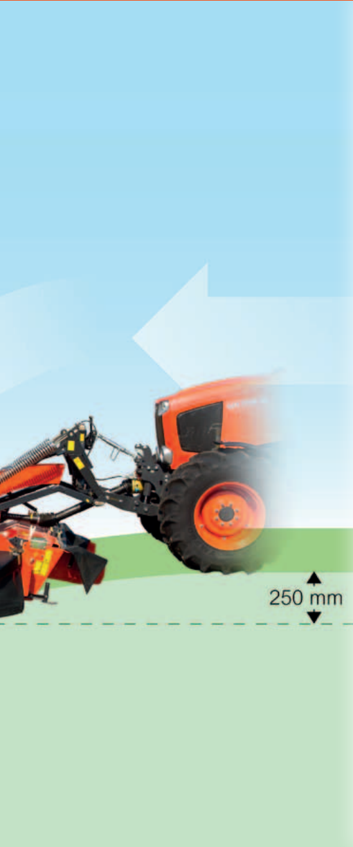
Vertical adaptation of 24° to adjust to uneven fields.
