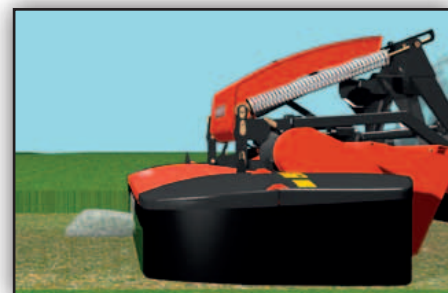
The suspension design protects the cutterbar against foreign obstacles.
