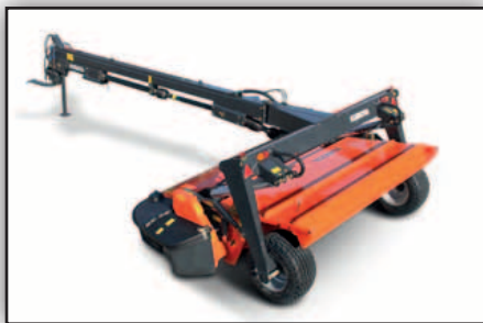
DMC8500T series – centre pivot trailed mower conditioner with steel tine or roller conditioning and 3.2-3.5m working width.
